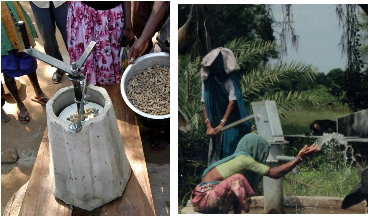
Figure 2: Appropriate Technology innovations designed and implemented by industrial designers. Concrete nut sheller (left) and sheet metal water pump (right).
