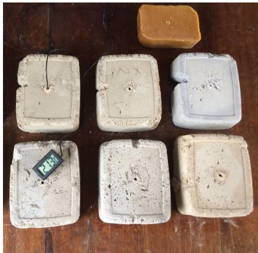
Figure 11: Left – block testing concrete and wax temperature insulation. Right – live hive temperature recording with concrete ad wooden hives.
