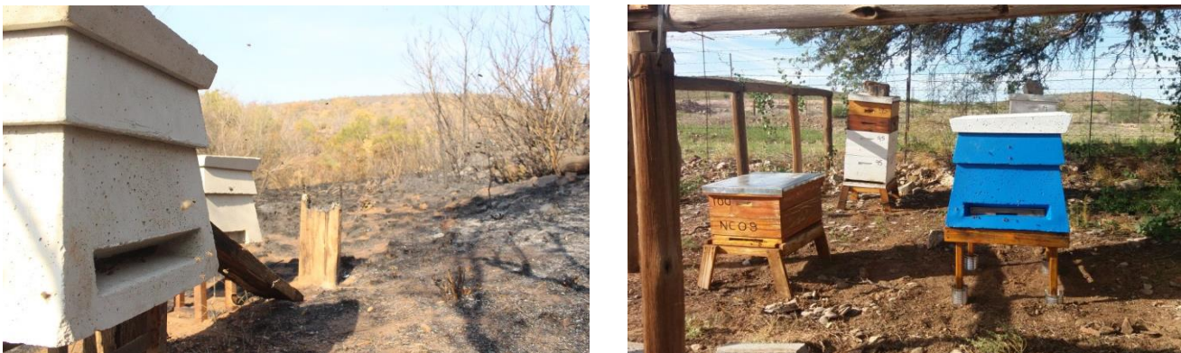
Figure 14: Ongoing field testing of lightweight concrete and wooden beehives.
