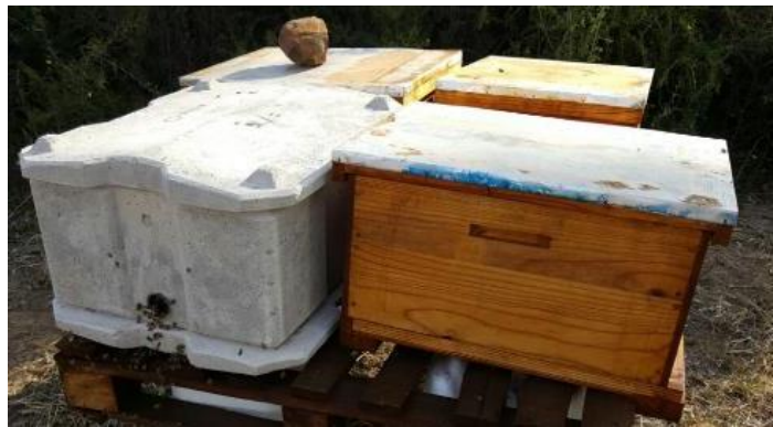
Figure 11: Left – block testing concrete and wax temperature insulation. Right – live hive temperature recording with concrete ad wooden hives.
