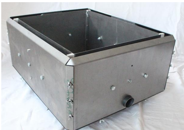
Figure 9: Left - Sheet steel beehive chamber. Right - unfired clay hive.
